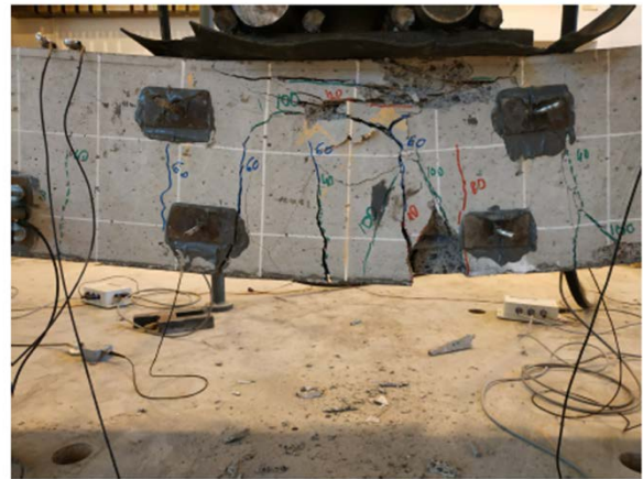
Figura 7. Crack pattern at failure of beam T6a.
