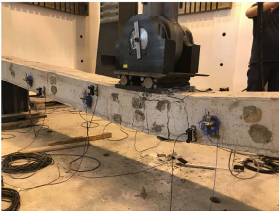
Figura 6. Crack pattern at failure of beam T4a.
